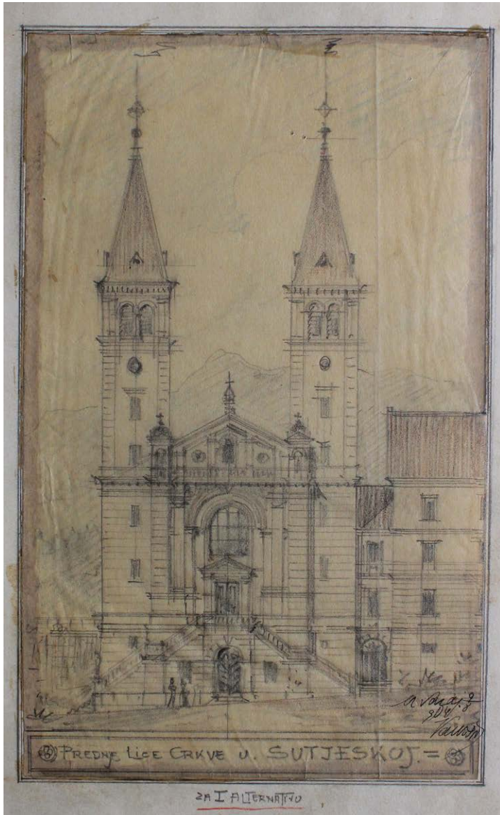
Figure 11. The Parish Church of Saint John the Baptist, Kraljeva Sutjeska: elevation view of the main façade from the south-east; a segment of one of the alternative preliminary projects done by Josip Vancaš, dated 9 th August 1904 37
