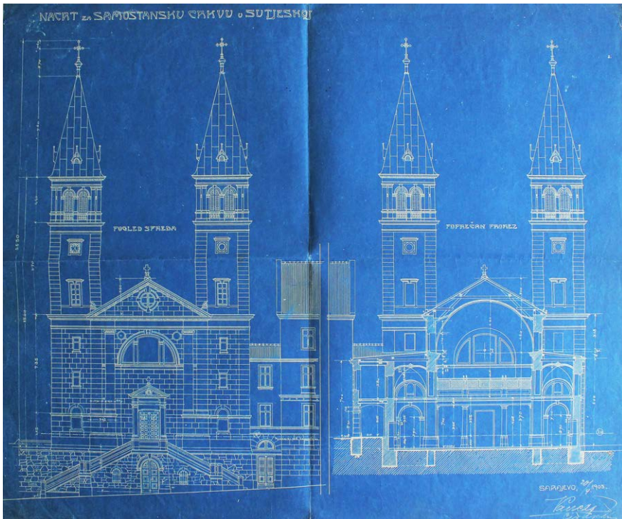
Figure 9. The Parish Church of Saint John the Baptist, Kraljeva Sutjeska: elevation view of the main façade from the south-east and cross-section through the central nave viewing the bell towers in the background; a segment of the second project done by Josip Vancaš, dated on 20 th April 1905 35
